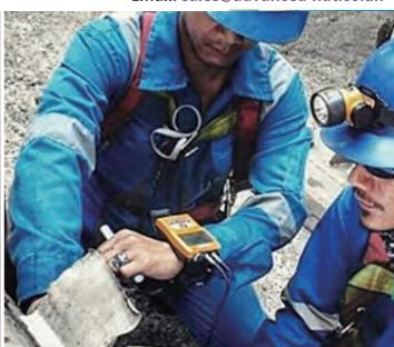
The CTS-30C is an entry-level & cost-effective thickness gauge, especially good for thru-coating thickness measurement on painted/ coated thin wall pipe in machinery, chemical, ship building, aeronautical and aerospace industries.
