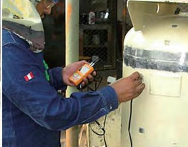
The CTS-30A/ CTS-30B ultrasonic thickness gauge, adopts micro-processor technology and advanced manufacture process design, can do measurement of thickness and acoustic velocity on metal and many different materials.
